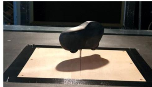
Figure: Velomobile on speed record run and scaled model velomobile in wind tunnel test.
