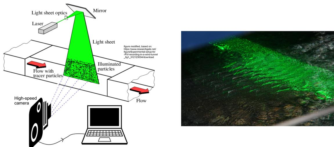
Figure 1: Left: Schematic of Particle Image Velocimetry setup. Right: A model of vegetation patch (e.g. group of glass blades) in a water flume illuminated by laser sheet for Particle Image Velocimetry.
