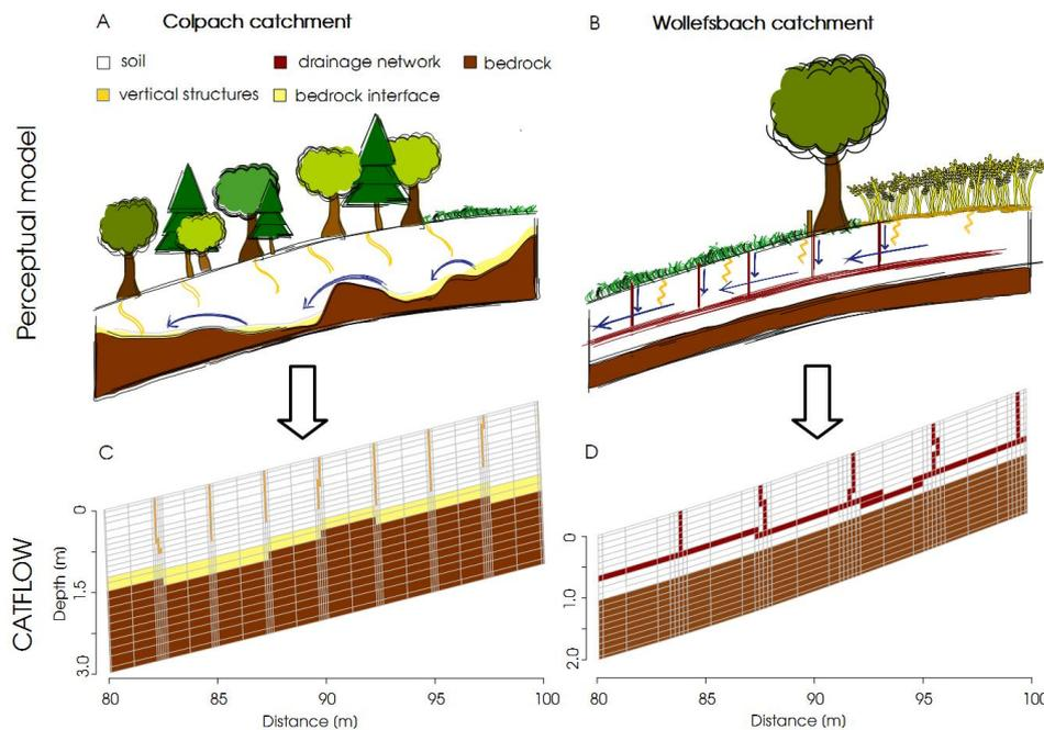
Figure 4: Perceptual models of the (a) Colpach and (b) Wollefsbach and their translation into a representative hillslope model for CATFLOW. It is important to note that only small sections of the model hillslope are displayed (C Colpach; D Wollefsbach).
